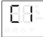
If the air conditioner is off, Auto clean starts immediately. If the air conditioner is running, Auto clean starts as soon as the air conditioner turns off.
