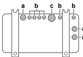
a Drain hole. Install a drain cap (2).
